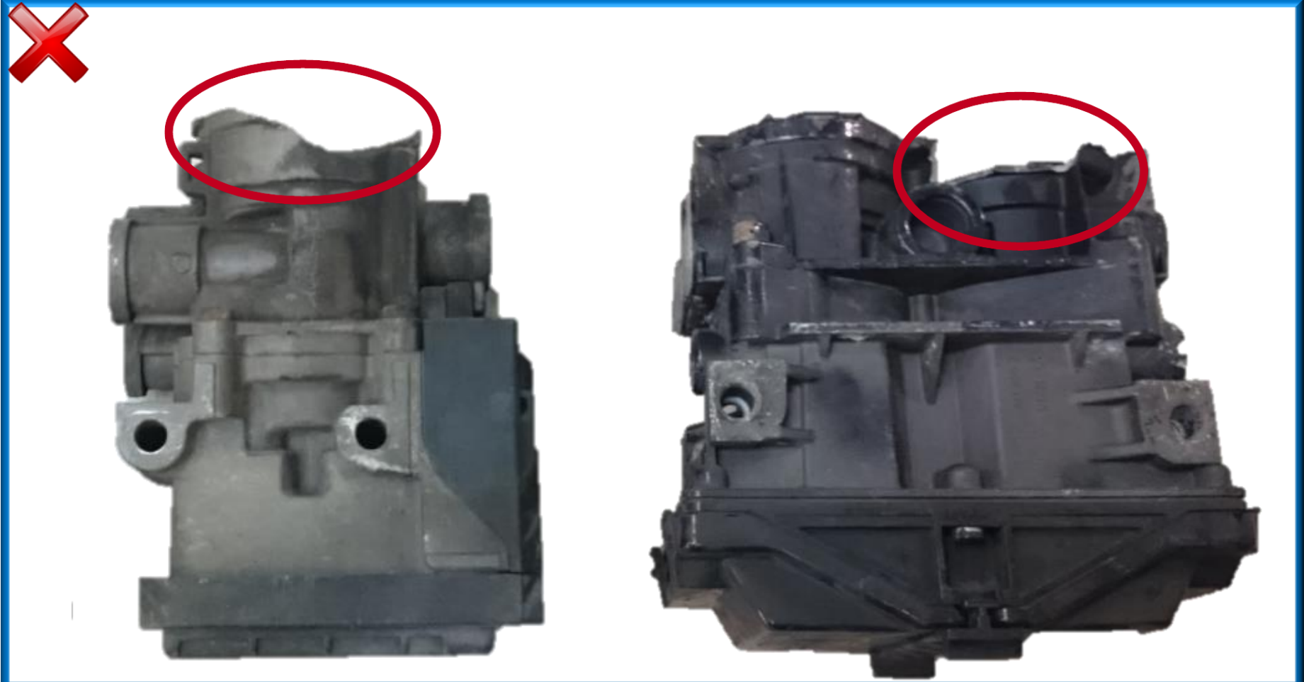
Heavily damaged housings caused by non-operational use
