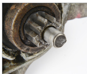
The rotor shaft and/or thread are badly damaged. The armature shaft is broken off or badly damaged.
