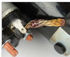
The unit is displaced or has been overloaded and has burnt out. The symptoms of this are: discolouration on the pinion, shaft and free wheel due to overheating. Burnt cable connection between solenoid switch and winding. The unit smells of burning.
