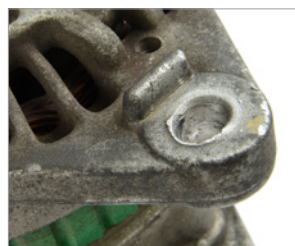
Enlarged/deformed attachment eyelet. Attachments have been broken off. Drive bearing shield of the starter is broken.
