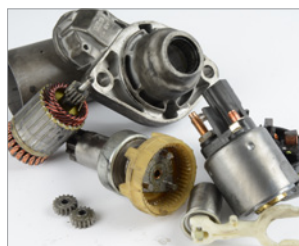
The unit is incomplete or disassembled into its individual parts. Parts are missing, e.g. regulator, pulley, vacuum pump on the alternator or armature, solenoid switch, windings on starter.
