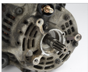
The unit is displaced or has been overloaded and has burnt out. The symptoms of this are: discolouration on the pinion, shaft and free wheel due to overheating. Burnt cable connection between solenoid switch and winding. The unit smells of burning.
