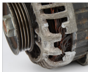
The unit is badly mechanically damaged or the housing is ruptured.
