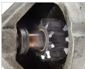
The unit is displaced or has been overloaded and has burnt out. The symptoms of this are: discolouration on the pinion, shaft and free wheel due to overheating. Burnt cable connection between solenoid switch and winding. The unit smells of burning.
