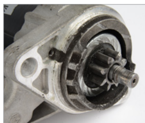
Enlarged/deformed attachment eyelet. Attachments have been broken off. Drive bearing shield of the starter is broken.
