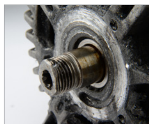
The rotor shaft and/or thread are badly damaged. The armature shaft is broken off or badly damaged.
