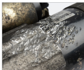
The unit is badly mechanically damaged or the housing is ruptured.
