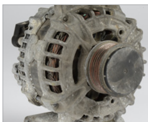
The unit is badly corroded/oxidised. The shaft is stuck or cannot be turned easily.
